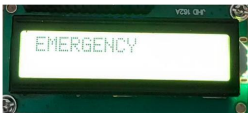
Figure 6. Emergency message displayed on the LCD
